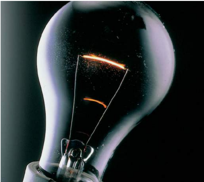
Figure 11.3 The metal filament in a lamp glows as the current passes through it. It also feels warm. This shows that the lamp produces both heat and light.
