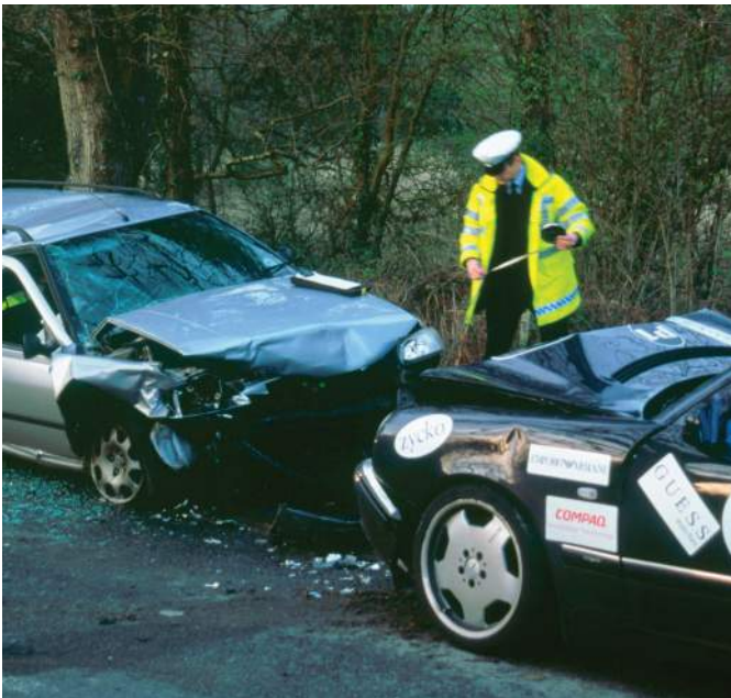
Figure 6.7 The front of each car has crumpled in, as a result of a head-on collision.
