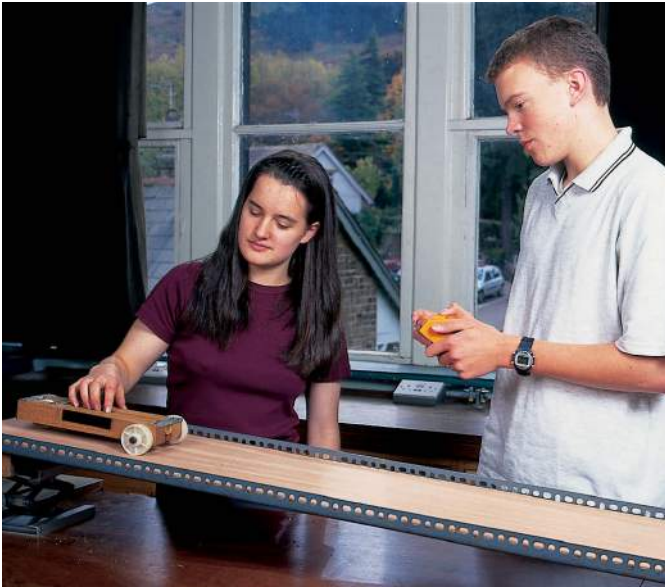
Figure 4.9 These students are investigating the acceleration of a trolley down a sloping ramp.
