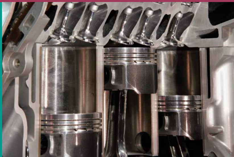
Figure 19.1 The pistons inside this car engine oscillate up and down as the engine powers the car.
