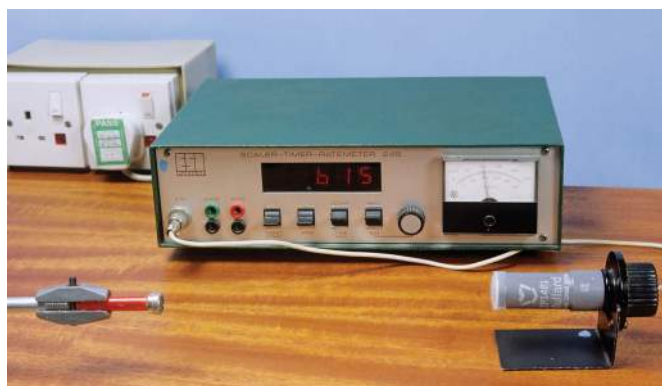
Figure 31.7 The time constant of this ratemeter can be adjusted to smooth out rapid fluctuations in the count rate.
