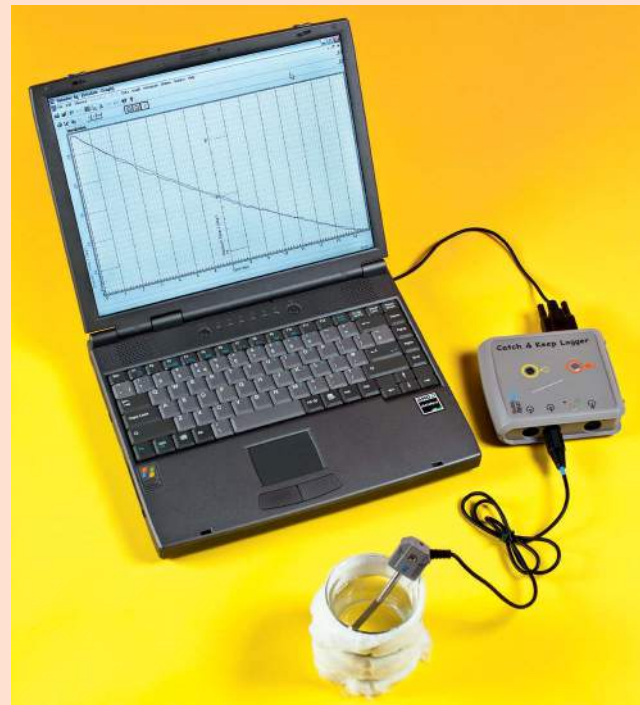
Figure 25.11 Using a datalogger to investigate the characteristics of a thermistor in a potential divider circuit. During the experiment, the screen shows how temperature and output voltage change with time. After the experiment, the same data can be displayed as a graph of p.d. against temperature.
