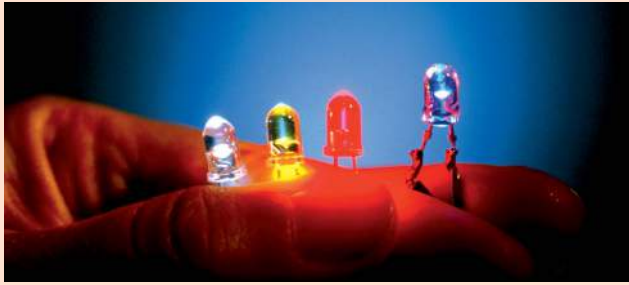
Figure 30.5 Light-emitting diodes (LEDs) come in different colours. Blue (on the right) proved the trickiest to develop.
