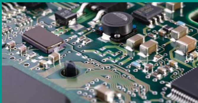
Figure 10.1 A complex electronic circuit – this is the circuit board which controls a computer's hard drive.
