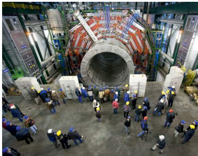
Figure 16.10 Particle accelerators have become bigger and bigger as scientists have sought to look further and further into the fundamental nature of matter. This is one of the particle detectors of the Large Hadron Collider (LHC), as it was about to be installed. The entire collider is 27 km in circumference.
