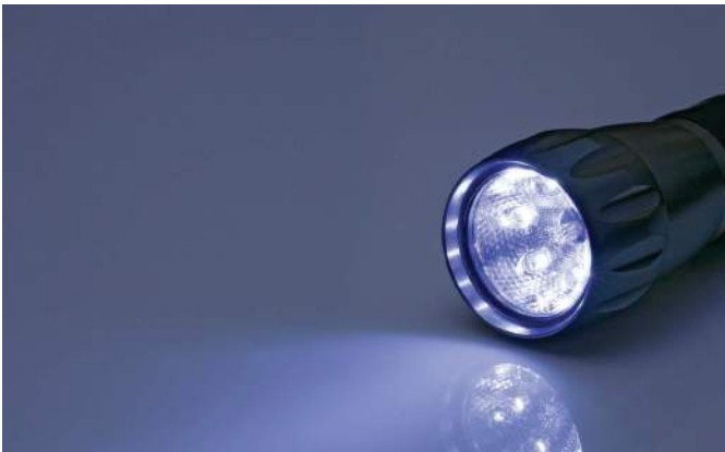
Figure 11.8 This torch has seven white LEDs, giving a brighter, whiter light than a traditional filament lamp.
