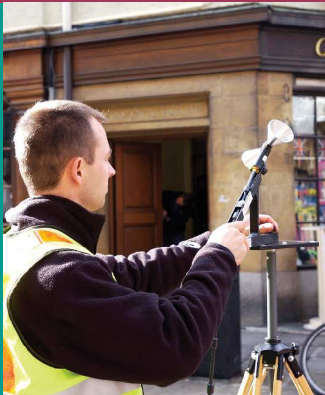
Figure 23.1 Mobile phone masts produce weak electric fields – this scientist is using a small antenna to detect and measure the field of a nearby mast to ensure that it is within safe limits.
