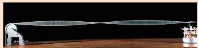
Figure 15.7 When a stationary wave is established, one half of the string moves upwards as the other half moves downwards. In this photograph, the string is moving too fast to observe the effect.
