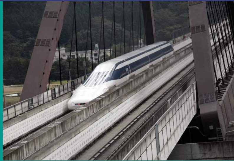
Figure 11.1 The Japanese JR-Maglev train, capable of speeds approaching 600 \text{ km h}^{-1} .
