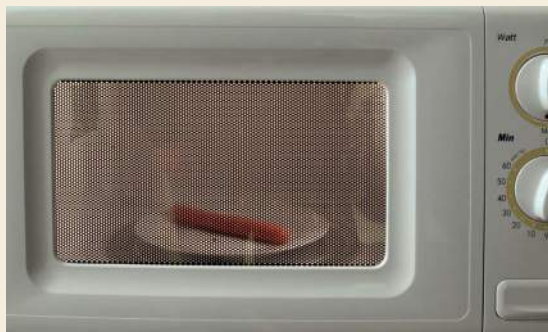
Figure 14.9 A microwave oven has a metal grid in the door to keep microwaves in and let light out.
