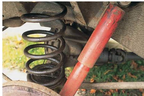
Figure 19.28 The springs and shock absorbers in a car suspension system form a damped system.
