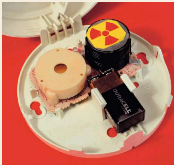
Figure 16.20 A smoke detector that uses the absorption of \alpha -radiation as the principle of its operation.
