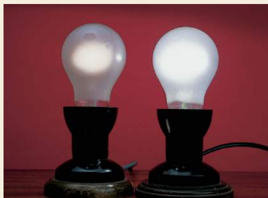
Figure 9.13 Both of these lamps work from the 230V mains supply, but one has a higher resistance than the other. For Question 13.
