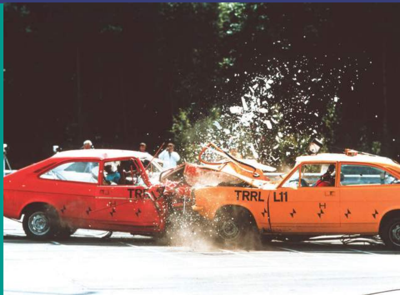
Figure 6.1 A high-speed photograph of a crash test. The cars collide head-on at 15 \text{ m s}^{-1} with dummies as drivers.
