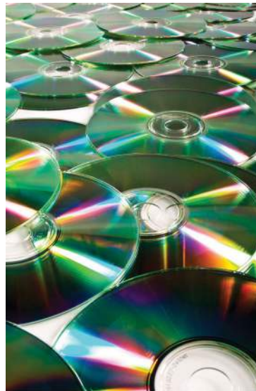
Figure 14.24 A CD acts as a reflection diffraction grating. White light is reflected and diffracted at its surface, producing a display of spectral colours.
