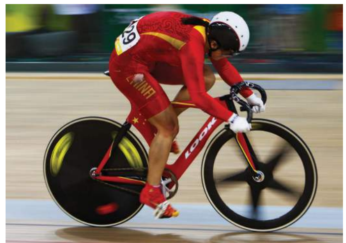
Figure 3.11 A racing cyclist adopts a posture which helps to reduce drag. Clothing, helmet and even the cycle itself are designed to allow them to go as fast as possible.
