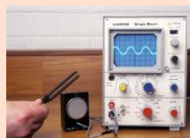
Figure 13.6 Measuring the frequency of sound waves from a tuning fork.
